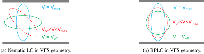
Fig. 2. Evolution of optical indicatrix in VFS cell geometry for nematic and blue-phase liquid crystals.
