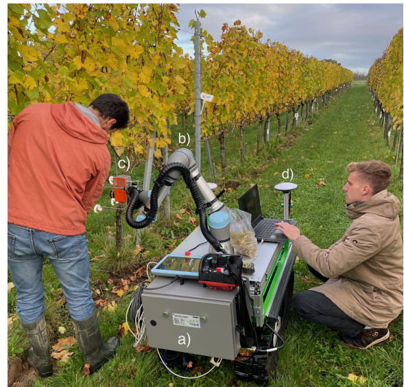
Fig. 1: The integrated IoT-enabled robotic platform during in-field data acquisition. Key components shown are a) the mobile robotic base, b) a collaborative robotic arm positioning the c) Specim FX10 hyperspectral camera, and d) the GPS antenna for georeferencing.
