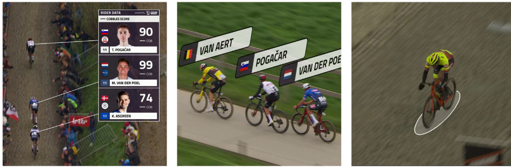
Fig. 1. Examples of augmented reality overlays applied to helicopter footage during cycling races. The static card overlay (left) displays rider data. The dynamic name card (middle) follows the rider’s movement and orientation. The ground marker (right) projects a visual indicator on the ground beneath the cyclist.
