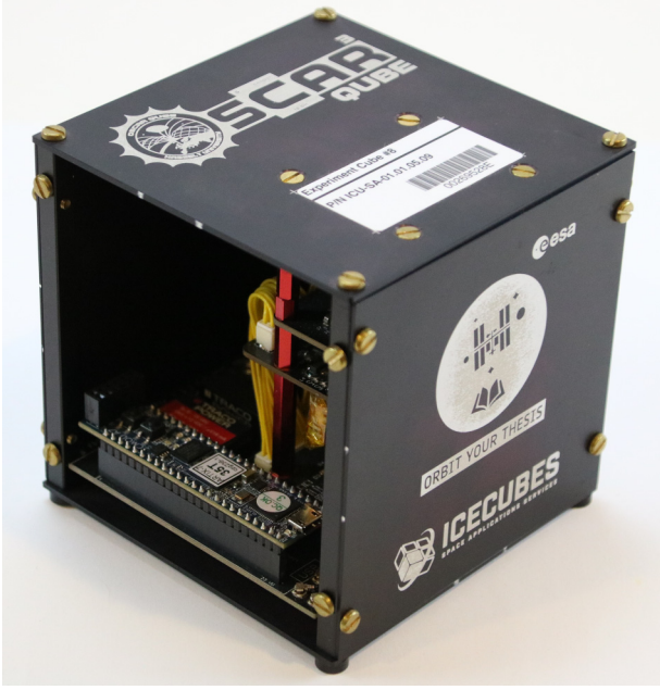
FIG. 4. OSCAR-QUBE diamond-based magnetometer flow board aboard the International Space Station.
