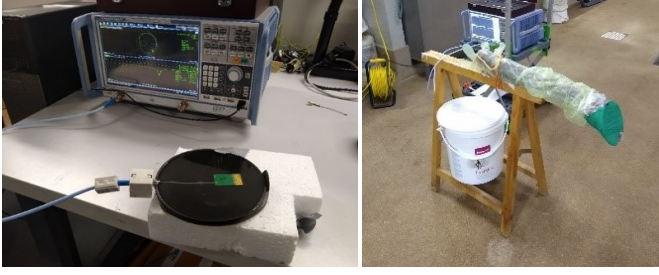
Fig. 4. The constructed pad (Left), the severed horse leg, covered in a hygienic veterinary glove. The part of the hoof is uncovered from the glove and the hoof pad is attached to it with tape. The cavity created between the hoof pad and the hoof is filled with Equi-pak. (Right)
