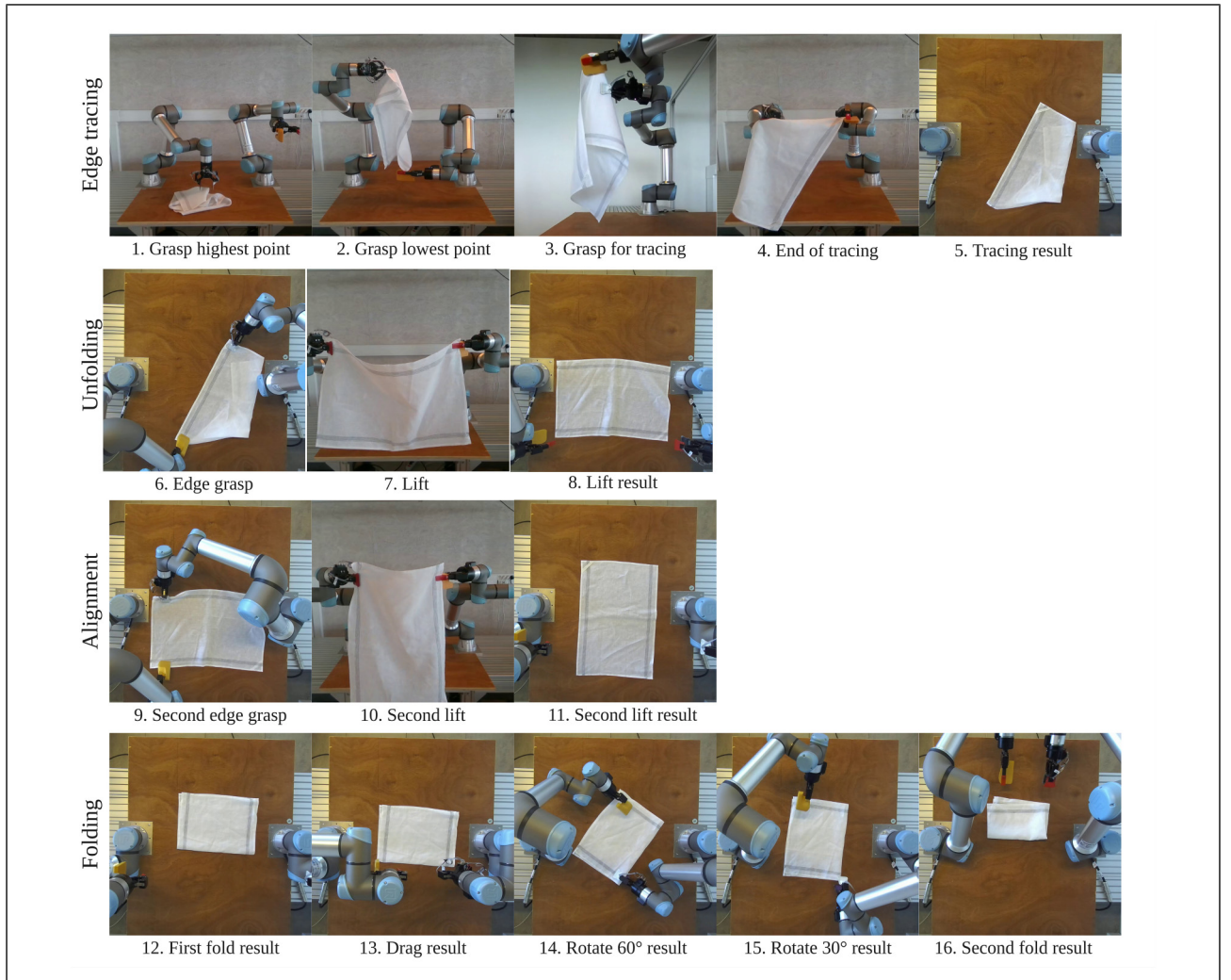
Figure 1. A typical run of the unfolding and folding pipeline shown as 16 key moments, grouped in four stages. Each row corresponds with a stage in the pipeline.
