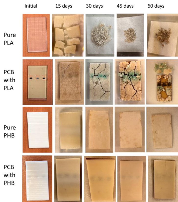
Figure 16. Images of solid fractions after biodegradation in compost at 0, 15, 30, 45, and 60 days.
