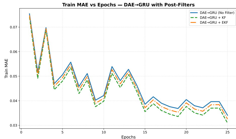
Figure 9. Training MAE versus epochs for DAE→GRU under No Filter, KF, and EKF configurations.
