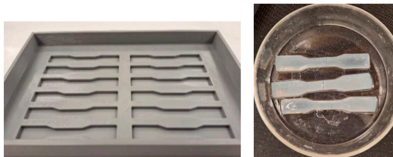
Figure 13. Dog-bone-shaped mold and sample for tensile test.
