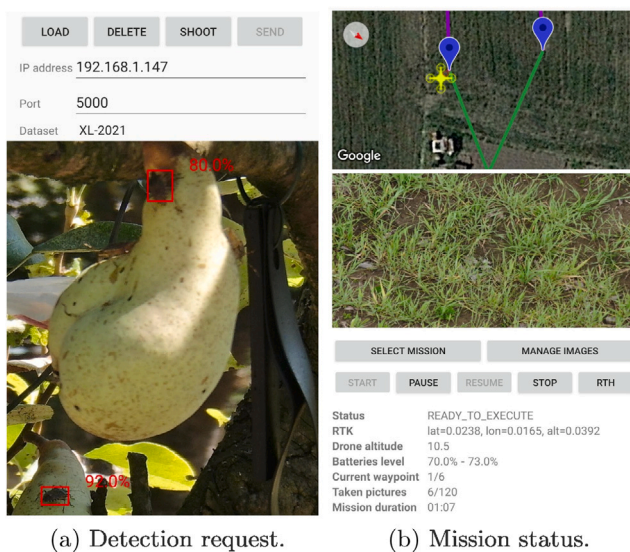
Fig. 5. Example of Android app interfaces. (a) Capturing new images or requesting a detection; (b) Status visualization of the ongoing autonomous mission.
