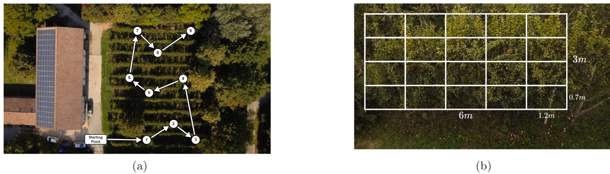
Fig. 6. Drone mission path (a); smart grid imaging technique (b).
