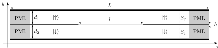
Figure 4: Geometry of the flying qubit interferometer. The width of the upper and lower channel is denoted by d_1 and d_2 , respectively. These 2-D channels are separated by a barrier with thickness h . A central scattering region of length l has a variable barrier height V_b and allows interaction between both channels. The channels are terminated on both sides by a PML. An electron originally in the lower channel (state |\downarrow\rangle ) will leave the channel in a superposition of |\uparrow\rangle and |\downarrow\rangle being both in the upper and lower channels with a given probability. The surfaces S_\uparrow and S_\downarrow , indicated with the dotted line, denote the planes through which the probability density current is calculated.
