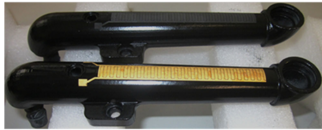
Figure 11. Laser structured MID (top) and metalized MID (bottom).
