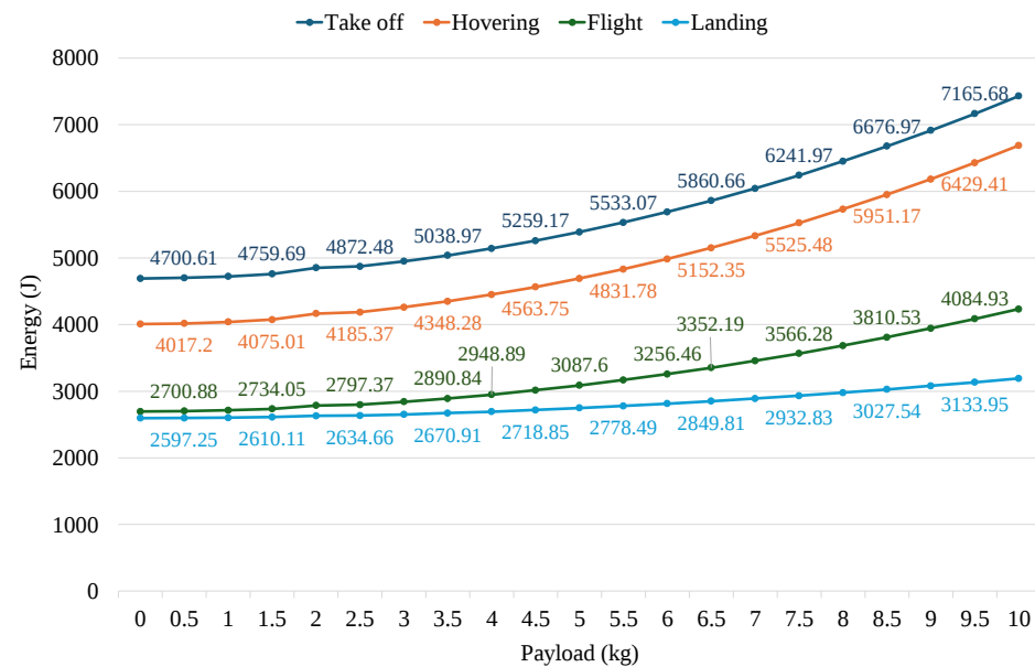
Figure 8. Energy consumption of UAV operations according to payload weight.
