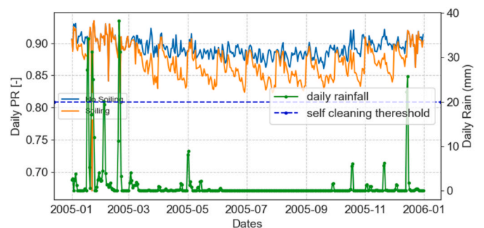
Fig. 15. Daily performance ratio without soiling (in blue) and with soiling (in orange). In green is the daily rainfall data and the dashed horizontal blue line indicates the cleaning threshold (i.e., daily rainfall equal or above 20 mm).
