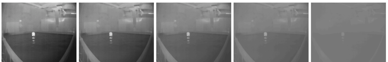
Fig. 11. Fog augmentation with progressive Meteorological Optical Range decay.
