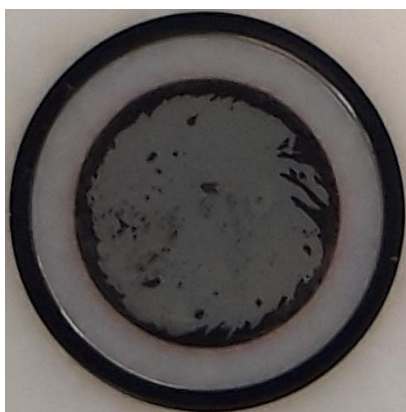
Figure S9: Digital photo of the RRDE after electroplating at 100 rpm in the dried electrolyte. In this case the procedure consisted of 3 steps; i) Cyclic voltammetry between 3.0 V and 0.1 V for 3 cycles (5 mV/s). ii) Galvanostatic plating at j_{\text{disk}} = -1 \text{ mA/cm}^2 for 742 s. iii) Relaxation at j_{\text{disk}} = 0 \text{ mA/cm}^2 .
