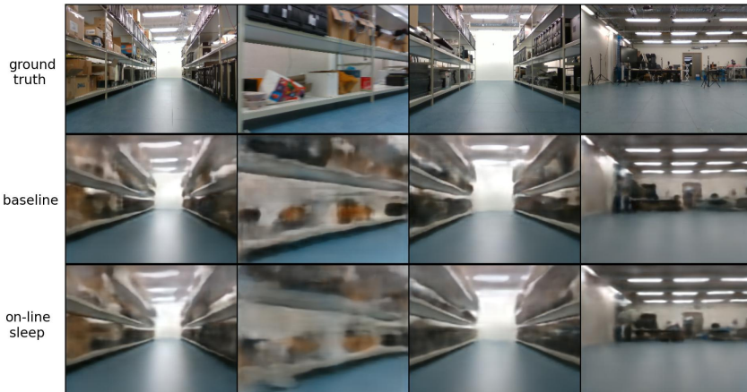
Figure 3.12: Reconstructed observations on the robot navigation environment. The top row contains ground truth observations, the second row contains reconstructions for a model trained with 128 latent space dimensions (achieving a reconstruction error of 9460), and the third row shows reconstructions for a model trained with on-line sleep with \tau = 12000 (see Figure 3.11).
