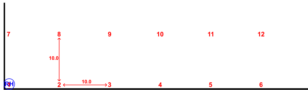
Figure 5. Locations of raster measurements. Blue label RH indicates antenna position. Dimensions are given in m.
