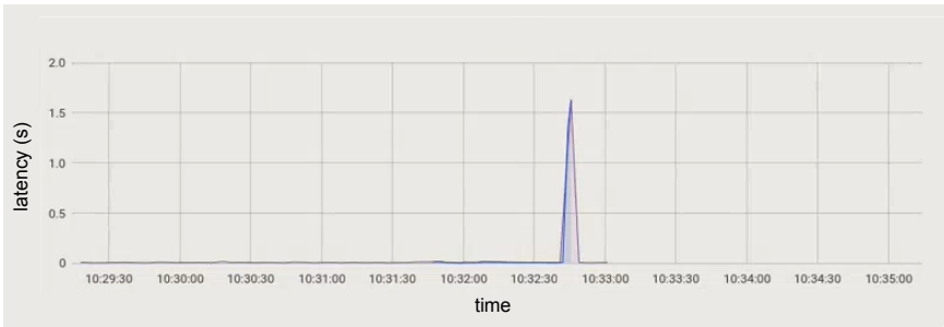
Figure 2.16: Grafana visualization of machine-control and iPerf traffic end-to-end latency with shared time slots
