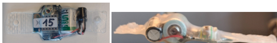
Figure 1. Tag containing UWB, IMU, and battery.
