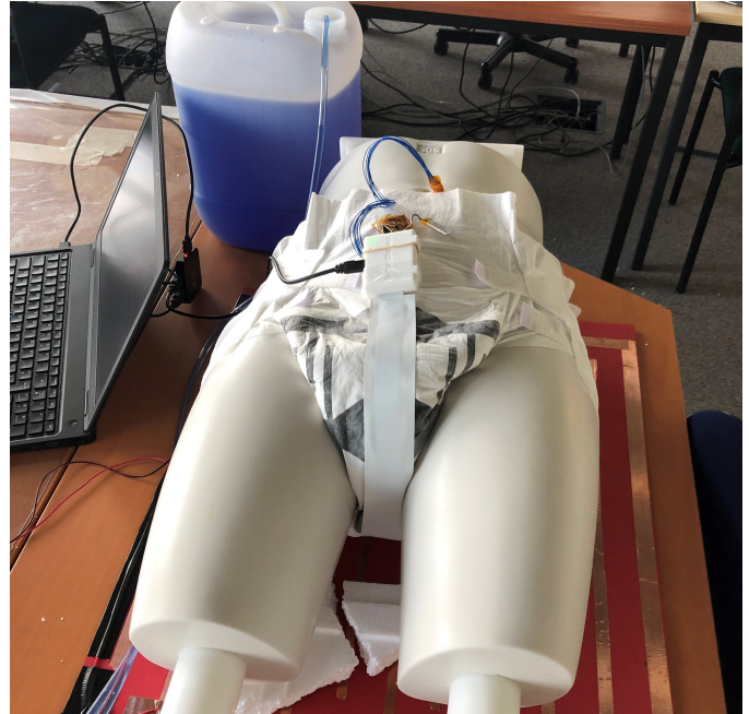
Fig. 8: Lab measurement on test dummy, with smart diaper, measurement strip, connected hardware interface and synthetic urine.
