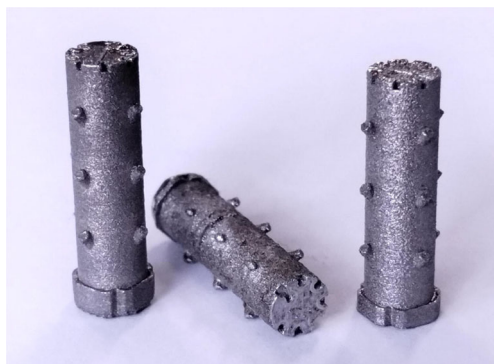
Fig. 1 Some samples used in this study. From left to right, a stainless steel 316L (CLM), a CoCr-DG1 (PLM), and a TiAl6V4 (CLM) sample
