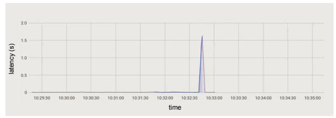
Figure 5. Grafana showing the machine-control and iperf traffic end-to-end latency with shared time slot
