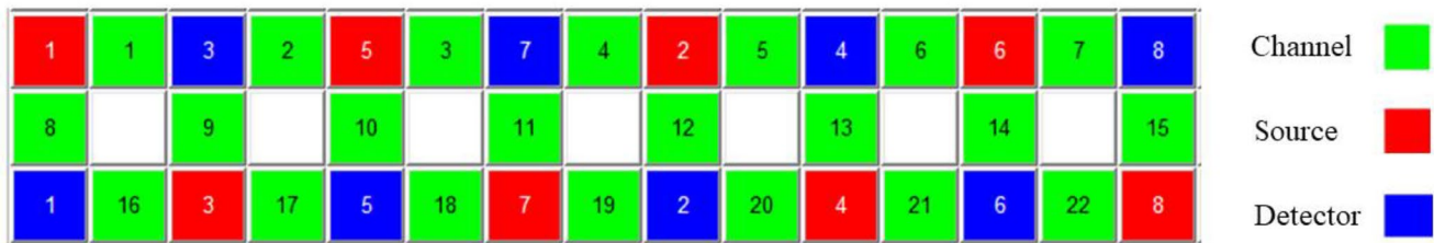
(a) Sensor layout for LIGHTNIRS device with a source-detector distance of 30mm
