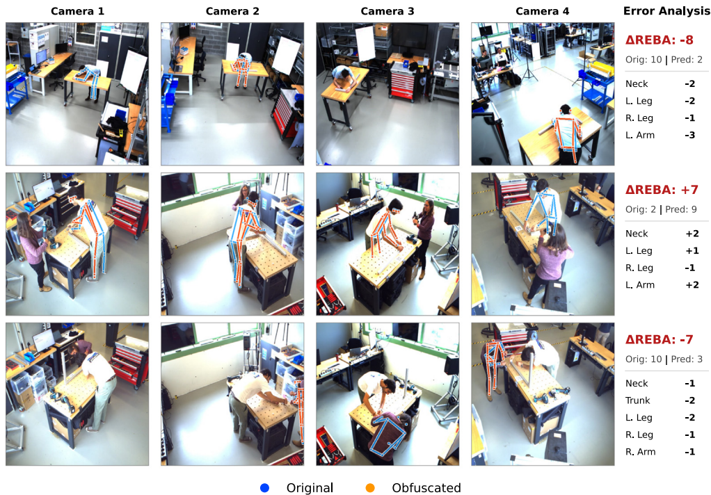
Fig. 17. Visualization of significant discrepancies between original and obfuscated REBA predictions. Each row corresponds to a single subject assessment. The obfuscated model predictions are overlaid on the original images for comparison.
