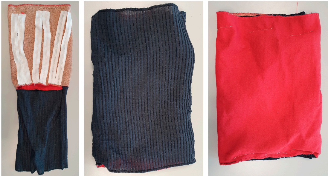
Figure 7. The washing tests for narrow fabrics and electronics integration were conducted in sleeve mock-ups.
