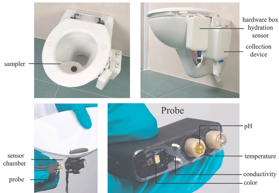
Fig. 1. The in-house-built prototype. This prototype consists of a hydration sensor and a collection device to automatically measure and collect the urine sample respectively. The probe is manually assembled with sensors to measure color, conductivity, pH, and temperature.
