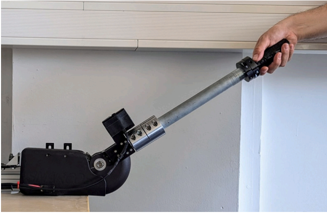
Fig. 10. Experimental setup for interaction experiment. A fixed reference position of 30^\circ is set, and the user interacts by moving the lever up and down at a fixed pace, trying to exert the same force throughout the experiment.
