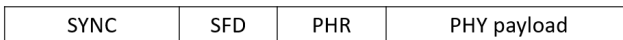
Figure A.5: Structure of a HRP UWB frame in the IEEE 802.15.4 standard.
