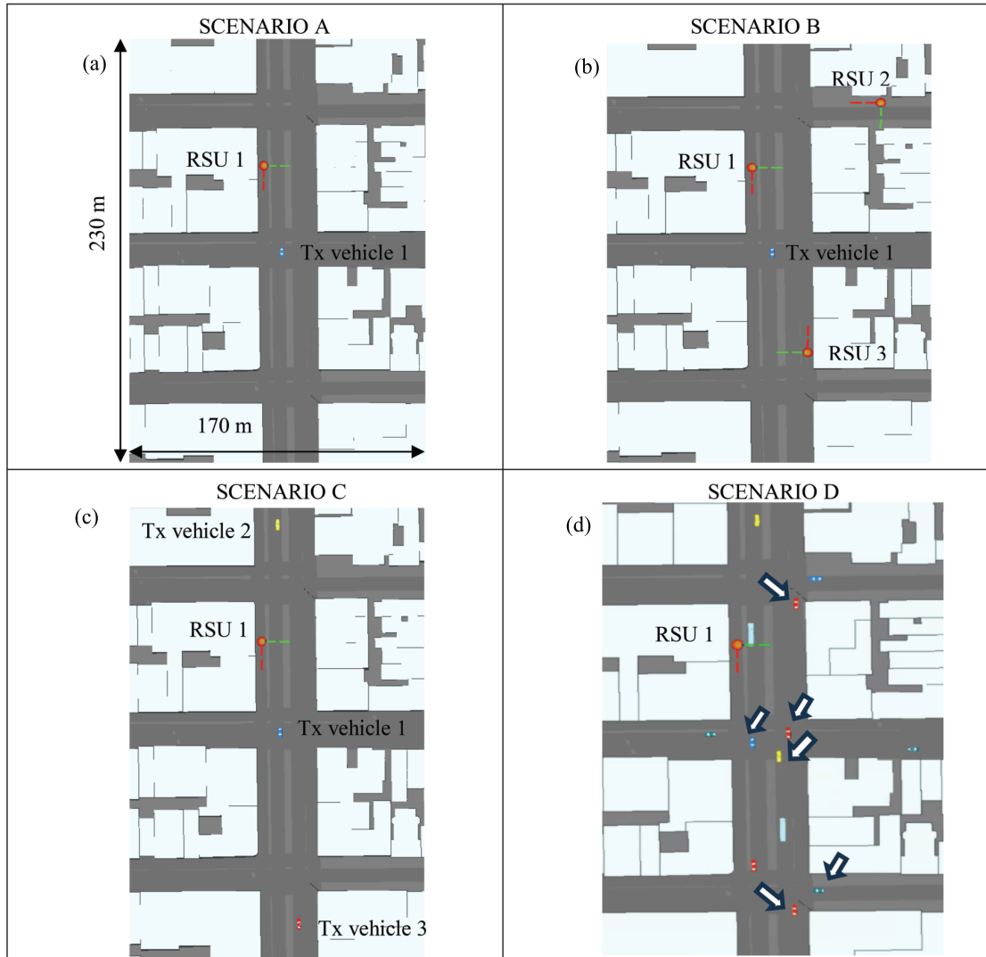
Fig. 2. Top view of the four different vehicular exposure scenarios investigated. (a) Scenario A has 1 transmitting vehicle (OBU) and 1 RSU. (b) In scenario B, in addition to the EM sources of scenario A, we introduced another 2 RSUs. (c) Scenario C, in addition to scenario A, has 2 more OBUs. (d) Finally, scenario D is the same as scenario A, with 4 more OBUs and 7 obstacles (cars and buses). The white arrows point to the vehicles that are transmitting, while the white blocks on both sides of the roads represent the buildings. Please note that the green and red lines at the RSU are the x -axis and y -axis, respectively.
