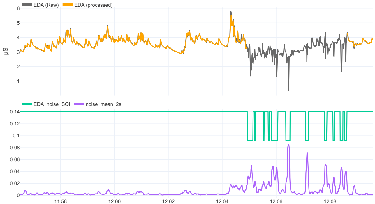
Figure 9. Skin conductance signal processing to discern valid and invalid regions and the resulting processed signal. The figure consists of two vertically stacked subplots that share the same x-axis. The upper subplot displays the raw EDA signal depicted by the gray line, with valid and invalid SQI regions distinguished by green and red backgrounds, respectively. The processed EDA data is illustrated by an orange line. Remark that there is no one-on-one relationship between the processed EDA data and the valid regions. This is because the duration and frequency of these invalid regions affect the eventual retention of the raw EDA signal. Specifically, brief and infrequent invalid segments, like those until 12h05, can be effectively imputed using interpolation, resulting in no data exclusion in the processed EDA signal. Conversely, as the frequency and/or duration of invalid segments increases, evidenced between 12 h 05 and 12 h 06, successful interpolation is compromised, resulting in disregarding these invalid regions. Moreover, processed EDA segments, but shorter than 60 s (e.g., valid segments between 12 h 06 and 12 h 08), are excluded given their limited analytical utility. The lower subplot elucidates the components of the skin conductance SQI. In alignment with the non-wear detection pipeline, multiple sub-SQIs are utilized. The noise amplitude of the EDA, averaged over a two-second window, is delineated by a purple line. This signal is thresholded to determine the noise sub-SQI, marked by the green line.
