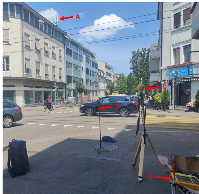
FIGURE 1 | Example of the measurement setup in Switzerland. The spectrum analyzer (D) was connected to the antenna (C) which was placed in line of sight of the base station (A). The UE (B) was placed in line with both the base station and the antenna of the spectrum analyzer, so that in the case of 5G technology (if present), the beam was directed towards the measurement setup.
