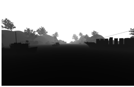
FIGURE 6. Example output from generated dataset. From left to right: bounding boxes generated automatically for vessels in the environment, depth camera measurements in grayscale (0 to 255m), segmentation map.
