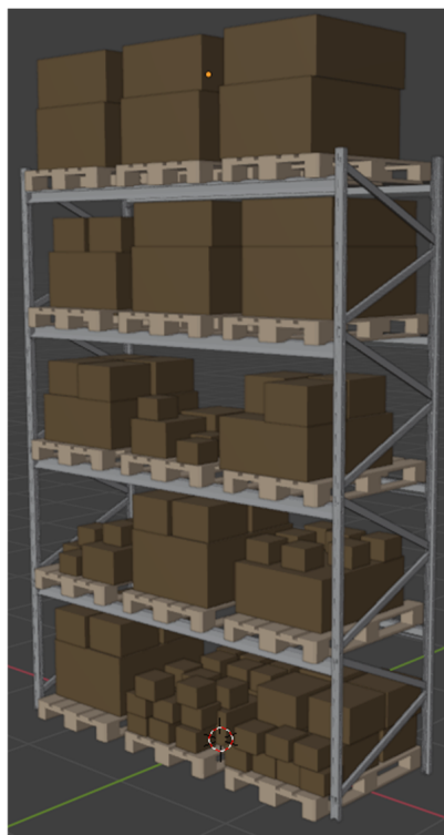
Figure 2. Detailed geometry of pallet racks modeled in Blender Ver 4.4. for MATLAB simulations. Wooden pallets carrying chipboard boxes of different sizes are arranged on metal frames.
