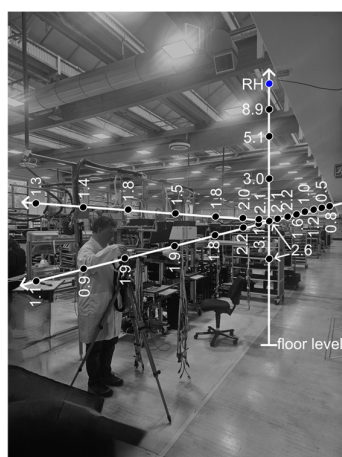
Figure 13. Extrapolated values of the measured electric field in the vicinity of a low-height pRRH in V/m. Measurements were taken at a height of 1.5 m in three directions at horizontal distances of 0.2, 0.5, 1, 2, 3, 4, and 5 m from the pRRH and directly below the pRRH at heights of 1, 1.5, 2, 2.5, and 2.8 m.
