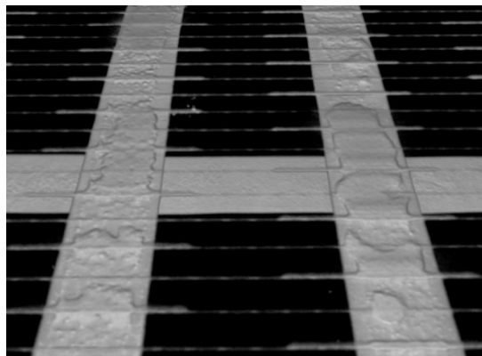
Fig. 7. Two parallel, 0.8 mm wide ribbons soldered to the cell metallization (fingers). The solder volume is slightly concentrated in the centre of the ribbons.
