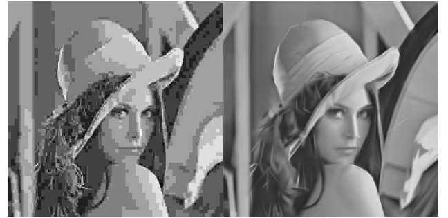
Fig. 4 JPEG (left) vs SMoE (right) - reconstruction at 0.15 bpp. At this low bitrate JPEG yields an image with heavy block artefacts. SMoE typically results in an image which is excessively blurred and with fine details missing.
