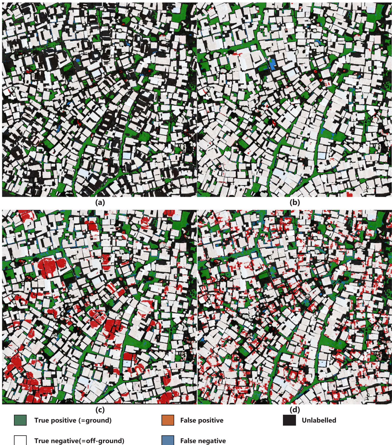
Fig. 6. Classification maps of the Dar es Salaam dataset for the rule-based training labels (a), FCN-RGBnZ (b), gLidar (c) and Lastools (d).
