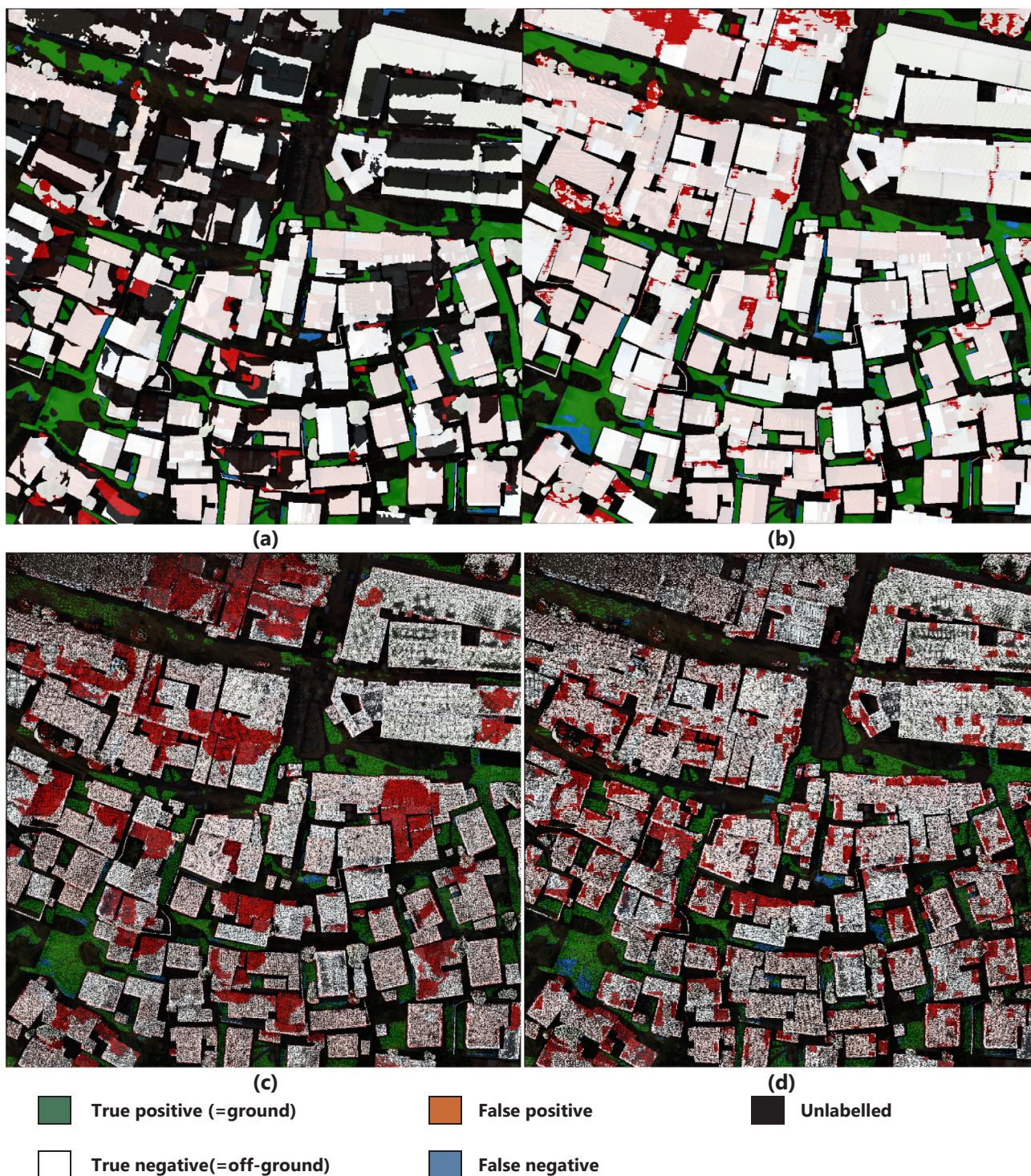
Fig. 5. Classification maps of the Kigali dataset for the rule-based training labels (a), FCN-RGBnZ (b), gLidar (c) and Lastools (d).
