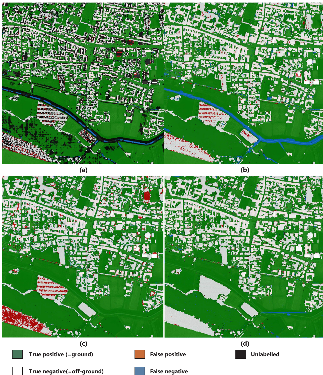
Fig. 7. Classification maps of the Lombardia dataset for the rule-based training labels (a), FCN-RGBnZ (b), gLidar (c) and Lastools (d).
