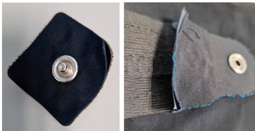
Figure 10. Degradation of lamination on electrode and the interconnect system samples.
