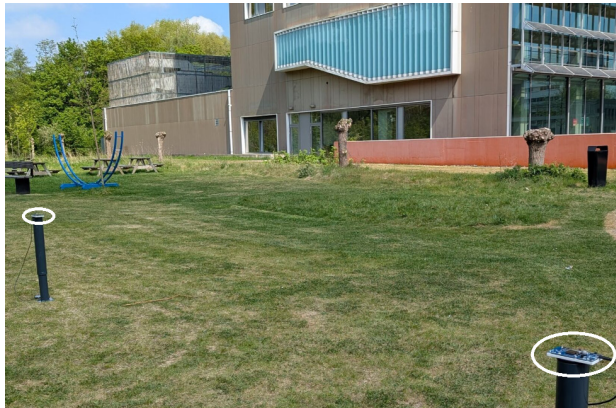
FIGURE 5. Example of outdoor measurement setup in which two BLE devices perform ranging.
