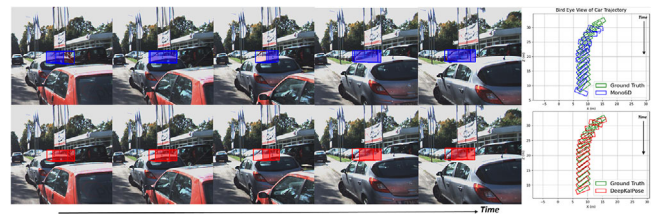
Fig. 4 Qualitative results demonstrating improved car trajectory estimation on an occluded and distant vehicle. The sequence displays the projected 3D bounding boxes: the upper row illustrates results from Mono6D [1], while the lower row illustrates results from our proposed methodology. The two figures on the extreme right detail the temporal bird's eye view (BEV) comparison between the 3D BB estimations by Mono6D and DeepKalPose, respectively
