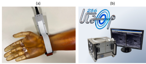
FIGURE 1. Setup for the experiment a) Array attached to arm phantom with Velcro band b) Ultrasound scanning system (ULA-OP 256).
