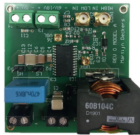
(b) Board 2: Texas Instruments LMG1210RVRT Si827GB-IS1 driver (GaNbridge and TI).
