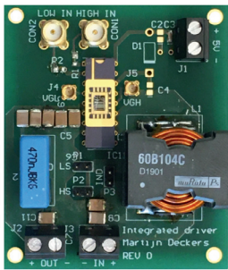
(a) Board 1: Imec integrated driver (GaNint).
