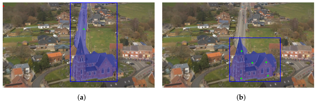
Figure 6. Example visualization of (a) the predicted SAM mask before refinement and (b) the predicted SAM mask after refinement using the POI recognition keypoint information.
