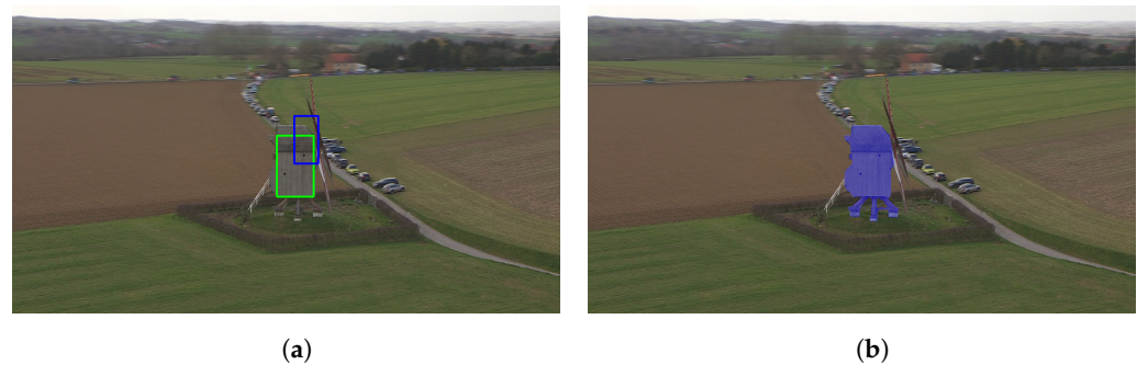
Figure 13. Visualization of the tracking results of the Vinkemolen at the middle of the broadcast time window using (a) the MedianFlow tracker (green box = ground truth, blue box = prediction) and (b) the SAM 2 tracker (blue mask = prediction). MedianFlow lost track of the windmill because the helicopter was rotating around it. In contrast, SAM 2 handles this rotation perfectly.
