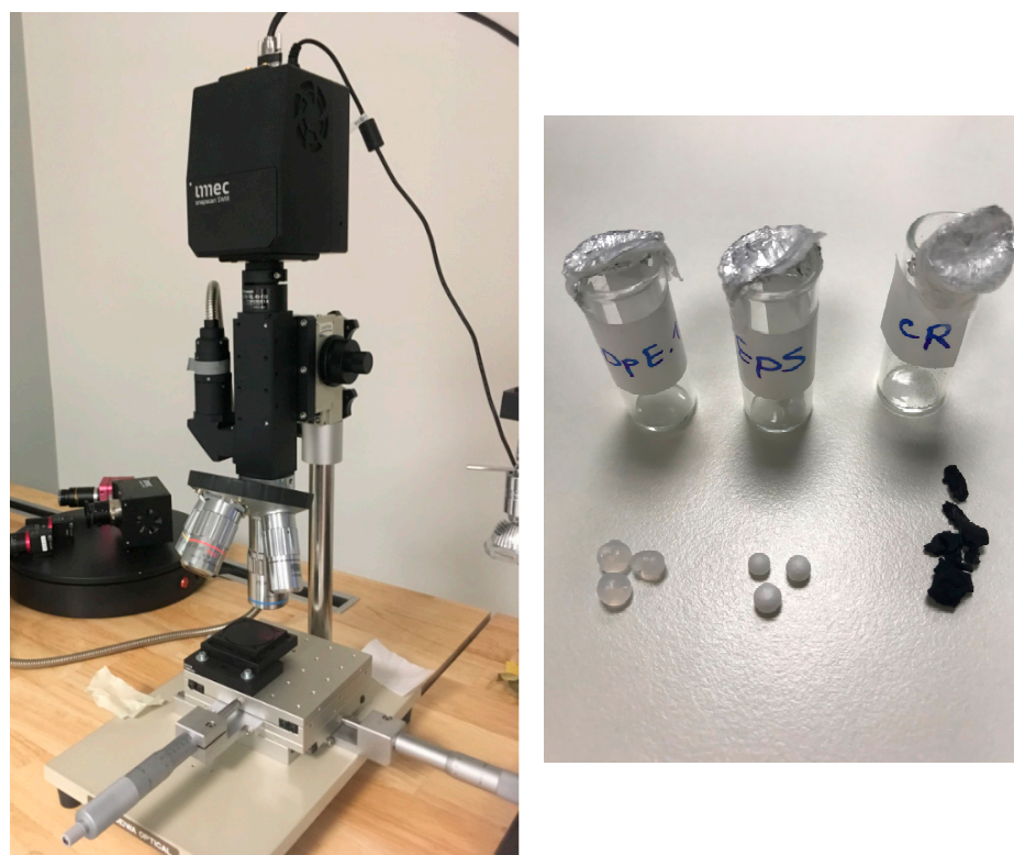
Figure 1. SnapScan SWIR camera with reflectance microscope (left) and plastic pellets (right).
